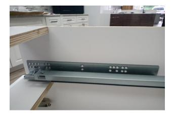
Step 9: Level Drawer Face using adjusting nob on Under Drawer Slide Clips as needed
