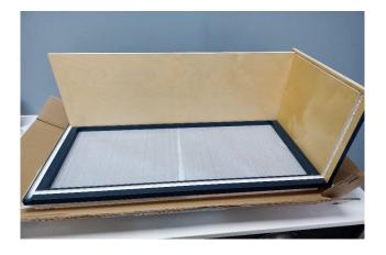
Step 4: Place remaning side panel top/bottom panel and back panel in grooves
