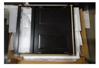
Place 2 Side Panel in Face Frame grooves -Step 2: Use nail gun or L-Bracket and Locking Plate where installed
