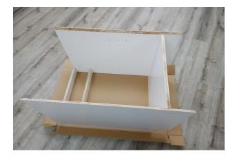
Step 4: Attach Back Panel with Bottom Panel in groove - Should fit snug and flush
